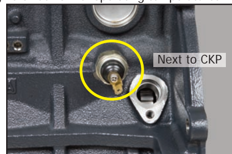
2.0L BETA 2004.5 - Present Spectra (LD) 2005 - Present Sportage (KM) 35.5 PSI @ 1500 RPM
