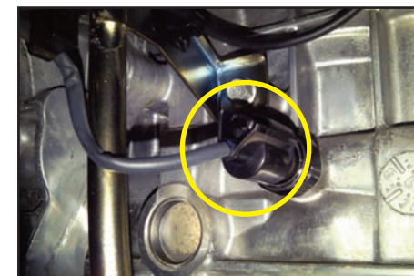
2.0L THETA II 2010 - Present Forte (TD) 15.6 PSI @ 1000 RPM
