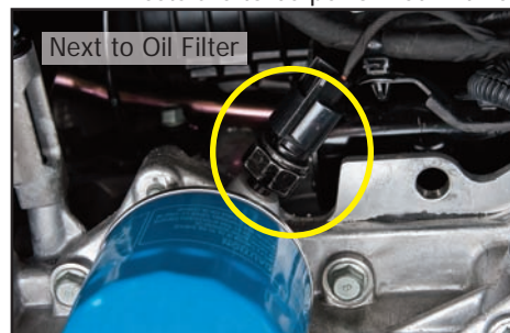
1.6L GAMMA 2010 - Present Soul (AM) 14.5 PSI @ 800 RPM
