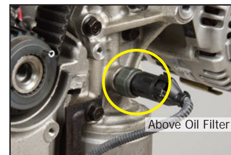
2.7L MU 2006 - Present Optima (MG) 2007 - Present Rondo (UN) 18 PSI @ 1000 RPM
