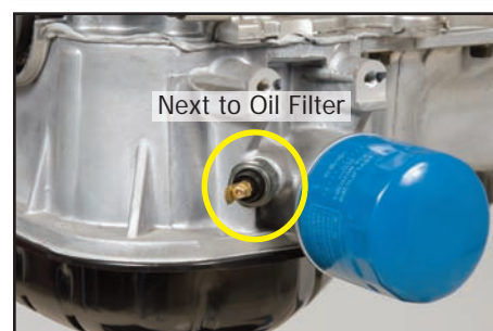
2.7L DELTA 2001 - 2006 Optima (MS) 2005 - 2010 Sportage (KM) 11.4 PSI @ Idle
