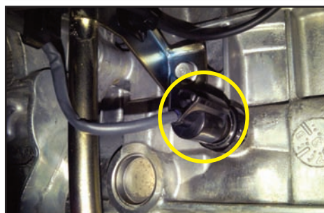
2.4L THETA II 2010 - Present Forte (TD) 2011 - Present Sorento (XM) 2010 - Present Optima (MG) 2010 - Present Rondo (UN) 2011 - Sportage (SL) 11.4 PSI @ Idle
