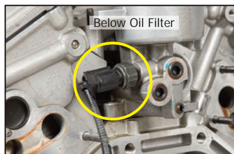
3.3L & 3.8L LAMBDA 2007 - Present Sorento (BL) 3.3L 2006 - Present Sedona (VQ) 3.8L 2007 - Present Amanti (GH) 3.8L 2007 - Present Sorento (BL) 3.8L 2009 - Present Borrego (HM) 3.8L 18.77 PSI @ 1000 RPM
